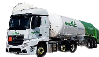
Figure 4: LOX tanker truck [26]
