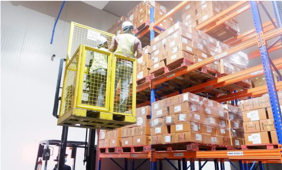
Figure 10: Forklift Access Platform
